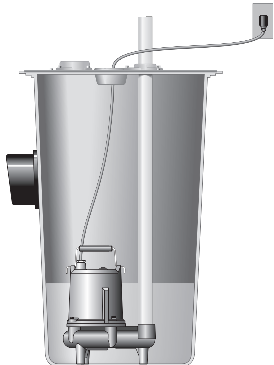
FIGURE 1 - SP40: TYPICAL INSTALLATION
