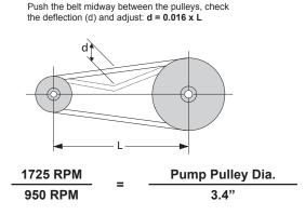
Solving this equation for the Pump Pulley diameter yields:
