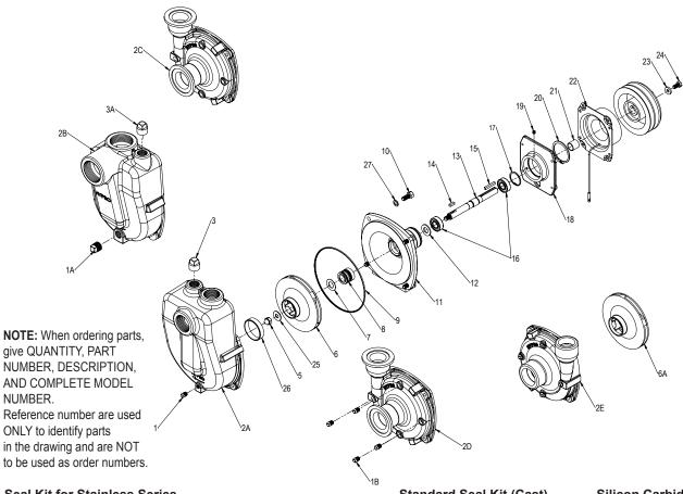
Seal Kit for Stainless Series No. 3430-0589 consists of: (1) Ref. 8 Mechanical Seal (1) Ref. 9 O-Ring
