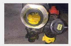
Pentair Hypro Express End Cap reduces chemical build up in the boom by reducing the "dead-ends" of pipe after the last nozzle body.
