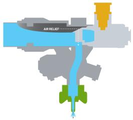
While in normal spraying operation, the valve is closed, pipe dead end is minimized and air is aspirated from boom to allow for faster nozzle body shutoff.
