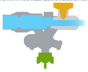
During flushing, valve is open and fluid is flushed out of the end of the boom. Push-to-Connect fittings are available to redirect flow to ground, bucket or tank.
