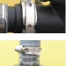
Improving safety through elimination of sharp edges that can harm operators.
