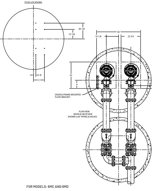
MIN. SUMP **PIPING** MIN. VALVE В C Α SIZE DIA. **BOX DIA.** 6" 3" 6' - 6" 5' - 6" 10-7/8 14" 3" 14" 6'-6" 6'-6" 10-7/8 7' - 0" 7' - 0" 10" 7-7/8 0" 11"
