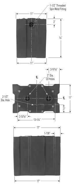
All dimensions in inches. Component dimensions may vary ± 1/8 inch. Dimensional data not for construction purpose unless certified. Dimensions and weights are approximate. On/Off level adjustable.
