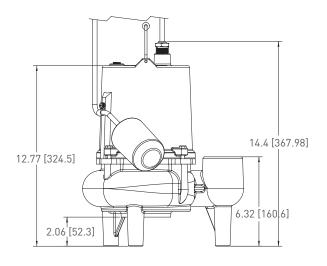
All dimensions in inches. Component dimensions may vary ± 1/8 inch. Dimensional data not for construction purpose unless certified. Dimensions and weights are approximate. On/Off level adjustable.
