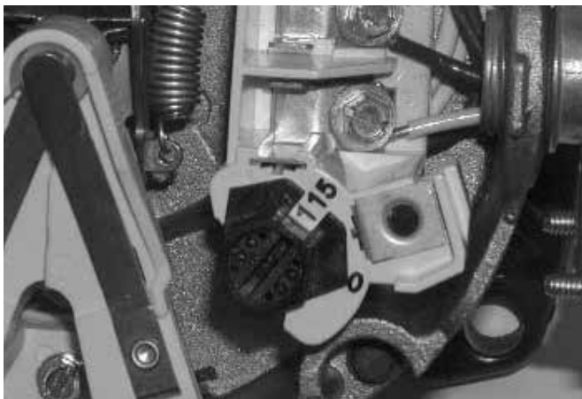
Figure 13: Motor Set for 115 Volt Operation
