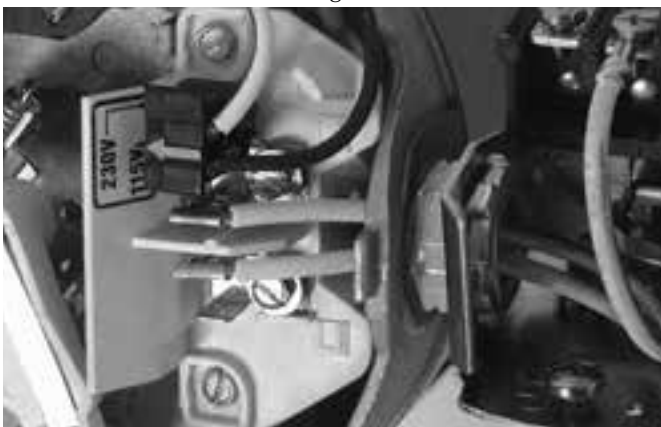
Figure 7: Voltage set to 115 volts, Plug Type
