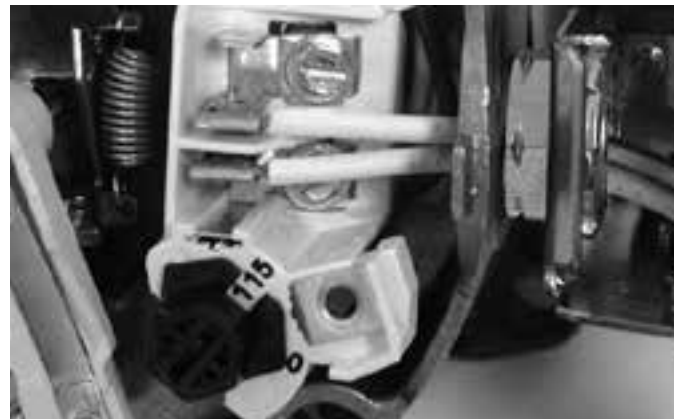
Figure 9: Voltage set to 115 volts, Dial Type
