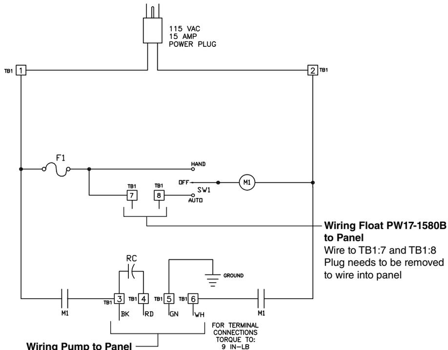
**Wiring Pump to Panel**
