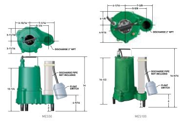
All dimensions in inches. Metric for international use. Component dimensions may vary  $\pm$  1/8 inch. Dimensional data not for construction purpose unless certified. Dimensions and weights are approximate. On/Off level adjustable.
