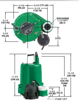
All dimensions in inches. Metric for international use. Component dimensions may vary ± 1/8 inch. Dimensional data not for construction purpose unless certified. Dimensions and weights are approximate. On/Off level adjustable.
