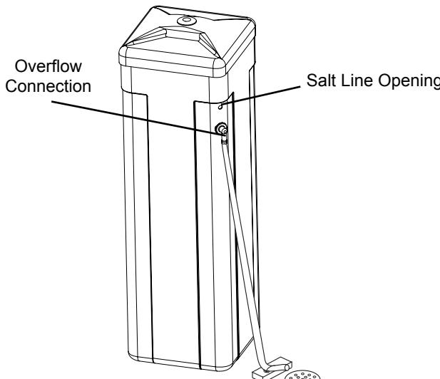
Figure 10 Tubing Connections
