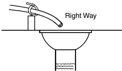
Figure 9 Drain Line Connection
