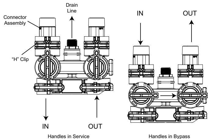
Figure 7 Bypass Operation
