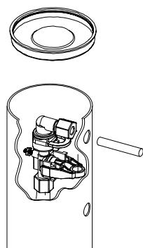
**NOTE: Once the tubing has been pushed into the nut it cannot be pulled out. The nut will need to be removed. See Figure 11 for correct assembly.**
