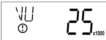
6. Press the Up button. Use this display to view the Reserve Capacity. This option setting is identified by "RC" in the upper left hand corner of the screen.
