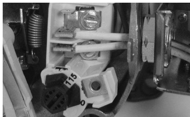
Figure 17 - Voltage set to 115 V, Dial Type
