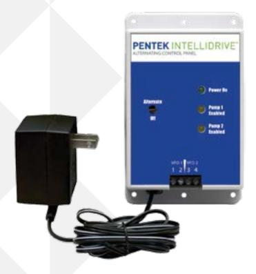
The Alternating Panel is designed to equalize wear on the pumps by alternating two Pentek Intellidrive VFD's every 24 hours. This panel alternates which pump is the lead and lag in a duplex system. It can also be used independently of the lead/lag function.
