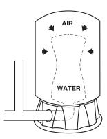
4. Water is being drawn from the tank: Compressed air in the tank forces water out of the separator.
