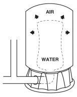
2. Water begins to enter the tank: separator as it fills with water.
