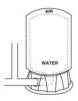
3. Pump-up cycle completed: Air is now compressed to the cut-off setting of pressure switch.
