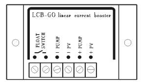
The SHURflo "LCB - GO" pump controller is a DC power converter designed as an interface between a DC (Solar)-Pump (e.g. SHURflo 9300 series) and a DC power source, like solar panels, wind generators,.. The main function of this controller is to maximise the daily water output while providing protection for the pump.
