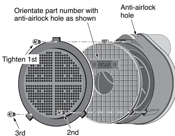
**Assemble Screen and Shield as shown.**
