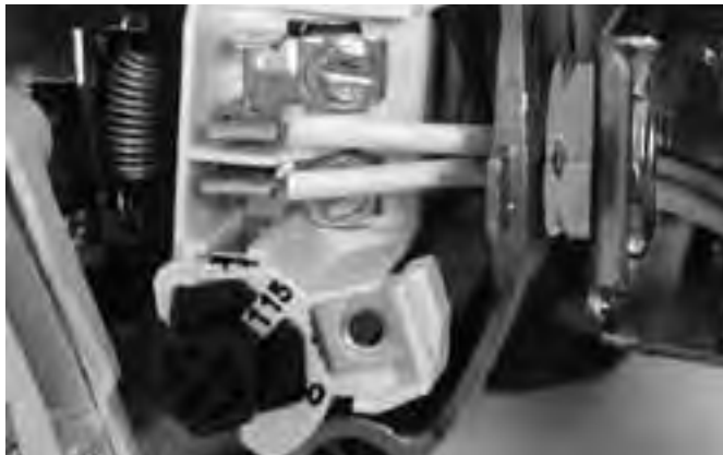
Figure 5: Voltage set to 115 volts, Dial Type
