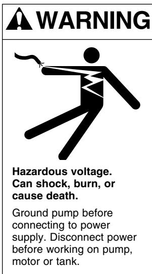
**⚠** Wire motor for correct voltage. See "Electrical" section of this manual and motor nameplate.
