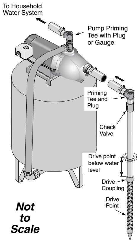
**Figure 1: Driven Point Installation**
