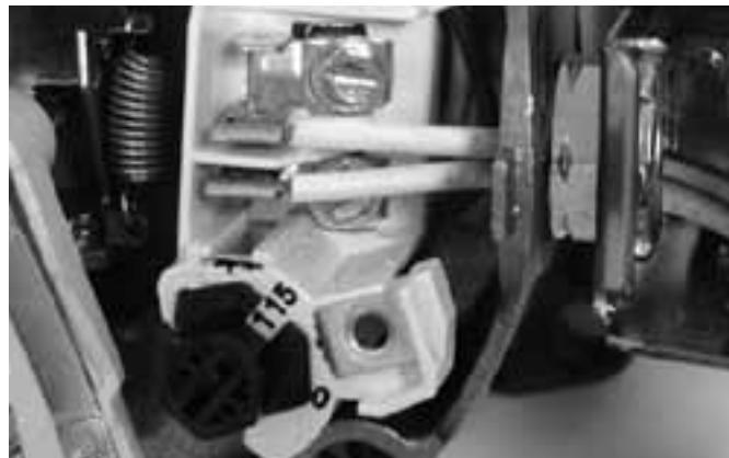
**Figure 7: Voltage set to 115 volts, Dial Type**
