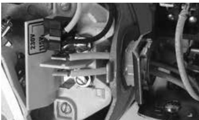
**Figure 6: Voltage set to 115 V, Plug Type**
