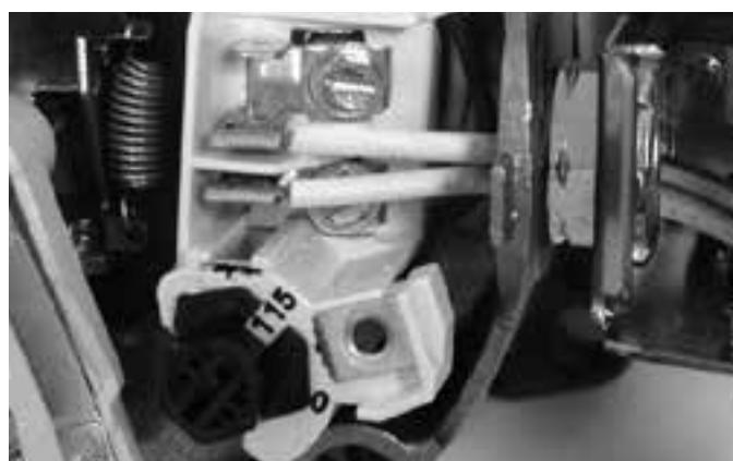
**Figure 8: Voltage set to 115 V, Dial Type**
