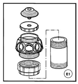
STEP 2 Assemble Hub, as shown, and insert assembly into flange opening.
