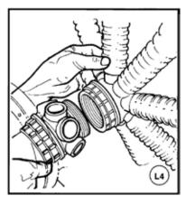
STEP 5 Hold Hub assembly with one hand and attach laterals as described in (step 3).
