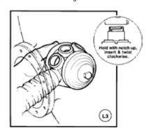
STEP 4 While holding Hub and lateral assembly No. 1, attach Hub assembly No. 2 with pipe attached and go to (step 5).
