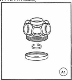
STEP 2 Thread cap onto Hub and insert through tank opening. (Holding Hub as shown).
