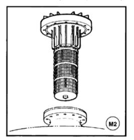
STEP 3 Using 1/2" wrenches, tighten 5/16" x 2-1/2" long bolts alternately, as shown, until the flange faces are flush with each other and seal is attained.
