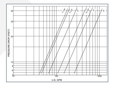
Calculate Required Pump TDH: [ A - B ] x 2.31 + C
