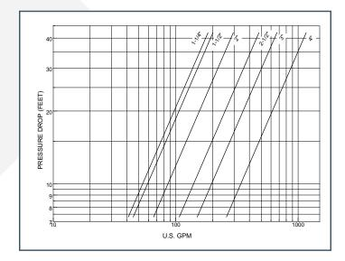
Calculate Required Pump TDH: [ A - B ] x 2.31 + C
