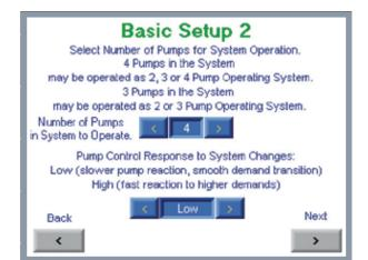
Easily configure the number of pumps in operation.
