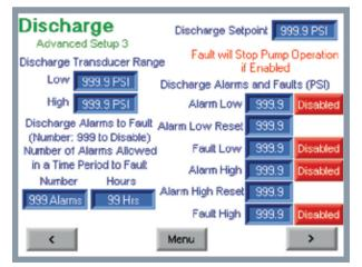
Determine your Alarm and Fault tolerances. Alarms will reset once operating conditions return to normal. Faults will cause the system to stop operating, resulting in operator assistance.
