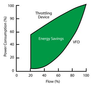
Figure 2. The amount of energy saved by using a variable frequency drive (versus a valve) to control flow
