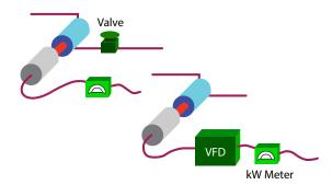
Figure 1. A mechanical throttling device versus a VFD
