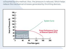
Applying a VFD to the pump allows control of the pump's speed electrically while using only the energy needed to produce a given flow. This is similar to applying a new pump with a smaller impeller. Figure 3 demonstrates the new pump curve and the energy
