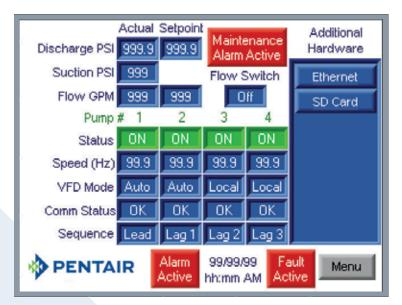
Realtime system operation, status, settings and hardware. Alarms, faults and maintenance indicators are active when set by operator.
