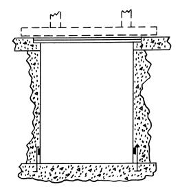
NOTE: Some larger size fiberglass basins are equipped with anchoring ridges near the bottom. Reinforcing rods or threaded bolts and washers may be used to help prevent floatation until the second concrete pour has set.
