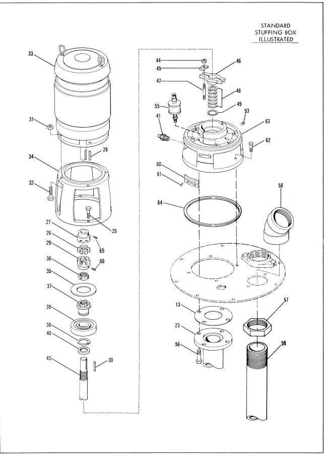
Figure 1. Model 631-632 Exploded View (Sheet 1 of 3)
