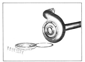
G. Capscrews, suction cover and gasket removed to expose impeller.
