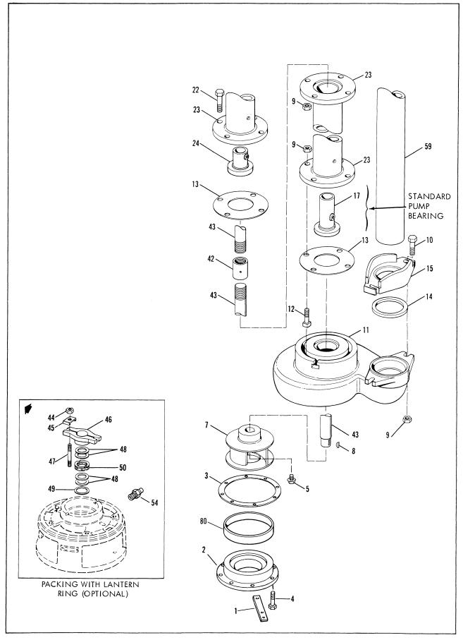
Figure 1. Model 631-632 Exploded View (Sheet 2 of 3)
