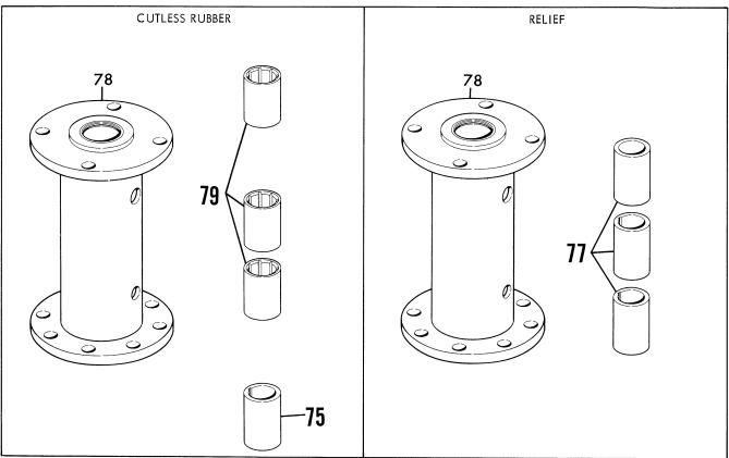
Figure 1. Model 631-632 Exploded View (Sheet 3 of 3)
