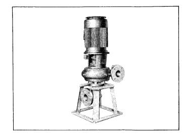
4. Unscrew capscrews (66B) to remove pump from base (21). The pump elbow (65) is removed by the loosening of capscrews (66). Gasket (64) may now be removed. If required, handhole cover (68) may be removed from elbow (65), by removing capscrews (69), nuts (69A), washers (69B) and gasket (67).
