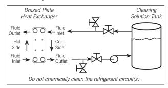
Do not heat the cleaning solution when back flushing through the heat exchanger. Flush the heat exchanger with fresh water after cleaning.
