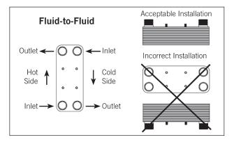
**Steam applications** – Unit should be installed in a vertical position to ensure the condensate drains from the heat exchanger.
