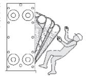
Transporting the plate heat exchanger: Before transporting the plate heat exchanger, always ensure that the hoisting gear is of sufficient dimensions and securely fixed. Never step underneath suspended loads.
