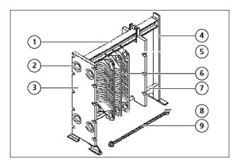
The plate pack consists of contoured heat exchanger plates (1) and the corresponding gaskets (2) of varying number and arrangement. Refer to the flow diagram for specific instructions as to the arrangement of the plates and gaskets in the plate pack.
