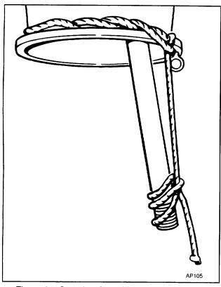
Figure 21. Securing Open Line Shaft Assembly
