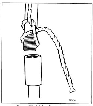
Figure 22. Joining Open Line Shaft
