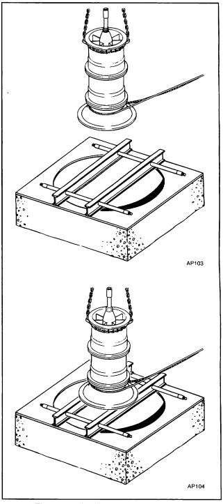
Figure 20. Positioning Bowl Assembly
