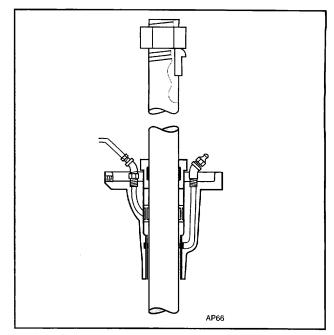
Figure 30. Packing Box Flush Provision
