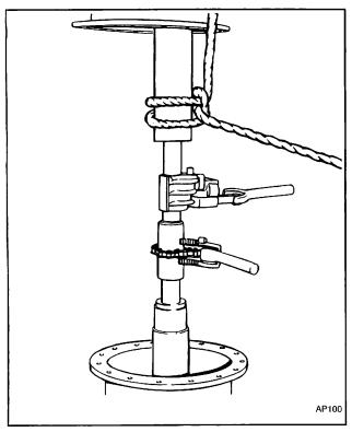
Figure 18. Connecting Enclosed Line Shaft Assembly
