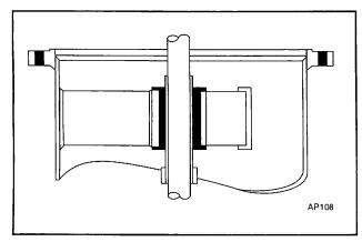
Figure 24. Open Line Shaft Bearing, Welded Configuration
