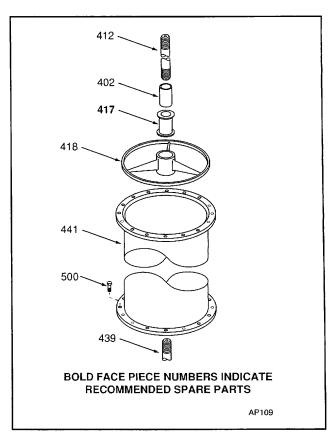
Figure 25. Open Line Shaft Bearing, Separate Configuration
