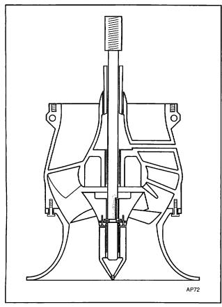
Figure 13B. Inspecting By-Pass Port - Mixed Flow Pump
