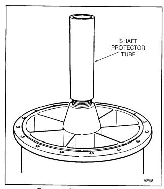
Figure 16. Shaft Protector Tube
