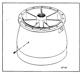
Figure 19A. Propeller Bowl Assembly - Mixed Flow Pump
