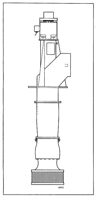
Figure 1A. Mixed Flow Low Lift Pump with Above Surface Discharge
