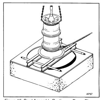
Figure 15. Bowl Assembly Resting on Beam Clamps
