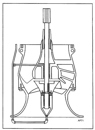
Figure 28. Bowl Assembly Lubrication (Mixed Flow Pump Illustrated)
