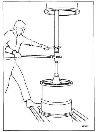
Figure 23. Connecting Open Line Shaft Assembly
