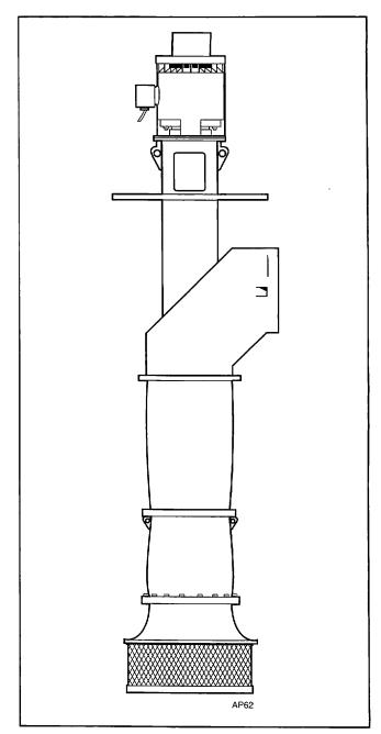
Figure 2B. Propeller Low Lift Pump with Below Surface Discharge
