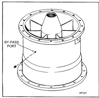
Figure 19B. Propeller Bowl Assembly - Propeller Pump
