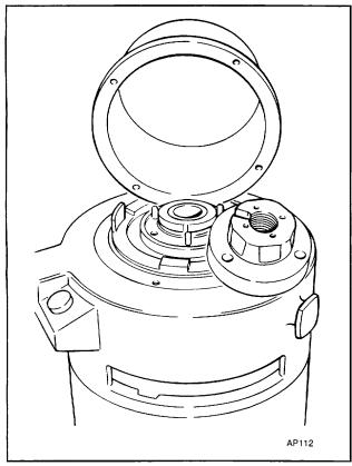
Figure 34. Removing Driver Canopy
