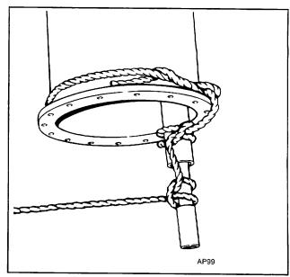
Figure 17. Securing Enclosed Line Shaft Assembly
