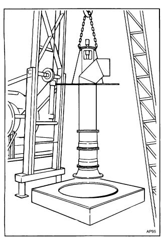
Figure 12. Raising Unit Over Mounting Position
