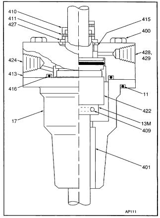
Figure 31. Typical Mechanical Seal -Ported for Flush System
