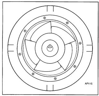
Figure 43. Mixed Flow Impeller
