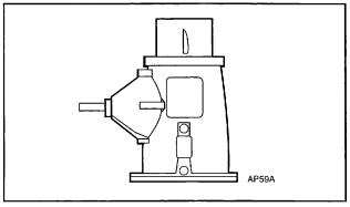
Figure 35. Right Angle Gear Drive
