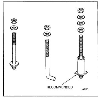
Figure 11. Foundation Anchor Bolts
