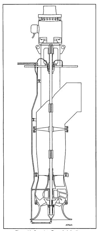
Figure 29. Complete Pump Lubrication - Open Line Shaft
