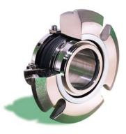
For split seals, the John Crane 3710 can be provided as an alternate to Chesterton's 442. The 3710 can only be used with 125#/150# flange ratings, and is only available for shaft sizes 1  $\frac{1}{2}$ " thru 2 7/16".
