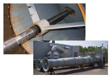
The upper rubber lineshaft bearing burned up on the sleeve, fell out of its retainer and slid down the shaft.
