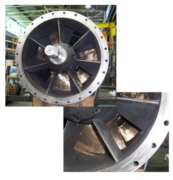
Discharge of the 500 HP two-stage 30P bowl assembly can be seen above. Once each bowl is complete, it is given a performance test. Then the rest of the pump including column, shafting, discharge elbow, and pedestal is assembled, painted, and ready for shipment. Pictured below are two-stage 24P and 30P bowl assemblies prior to testing.
