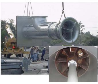
Many propeller pumps are used for drainage or flood control. Parson & Sanderson, who have represented Verti-Line for decades in Louisiana, sold two model 54P's. A new design for Verti-Line, they were driven by a diesel engine via right angle gear. These pumps help protect Ormond subdivision in Destrahan, LA, which is part of St. Charles Parish. Pictures courtesy of Jeff Leedy at Parson & Sanderson.
