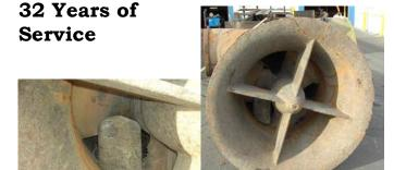
This Verti-Line 36P propeller pump was first installed 1974 for Manitoba in Water Stewardship in The Pas, Manitoba. Driven by a diesel engine via right angle gear, the pump operated until early 2006 when a rock was sucked into the impeller. Long time Verti-Line National distributor **Process** Equipment (formerly Wilron Equipment) in Canada pulled the pump for repair. Pictures courtesy of Mike McDonald at NPE.
