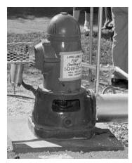
12", and only a 125# flange was available. With Verti-Line and Layne & Bowler under one roof after 1986, the WL head was offered to Verti-Line customers as the "LB" head. Very similar in both appearance and dimensions to Verti-Line's old AC head, consequently production of the AC head discontinued. Only the 25AC14 continued and was sold as the 25WL14.
