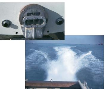
Providing the thrust was a Verti-Line 12FH bowl assembly powered by a Chevy 283 Hi-Po Corvette engine. Below is Walter McSweenie looking over the entire setup. Walter was manager of the foundry at Verti-Line.
