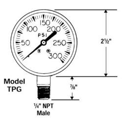
Case and Ring - Black coated steel Bourdon tube movement Socket - Brass ASME Type B -4 to 176°F (-20-80°C)
