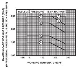
EXAMPLE: A model 1900 pump with a bronze casing has been selected for operating at a case working pressure of 240 psig at 150°F. Enter Table 2 at 150°F and read upward to 240 psig. It is determined that the selection is within the recommended maximum case working pressure area for 300 psi flanges and is therefore acceptable. Note that the example exceeds the maximum case working pressure unit if the material selected would have been 125 psi flanged cast iron or 150 psi flanged bronze.
