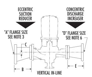
NOTE: Suction Reducers and Discharge Increasers for end suction fire pumps are the same dimensions as above.
