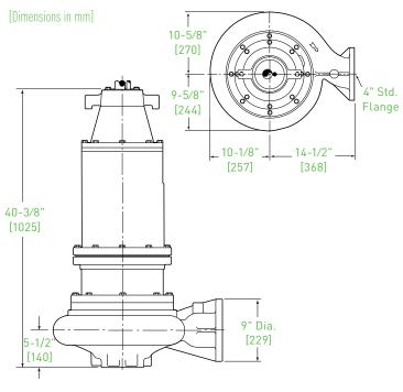
Pump performance is based on clear water (1.0 specific gravity @ 68°F) and pump fluid end (hydraulic) efficiency. Motor data based on 40°C ambient temperature.
