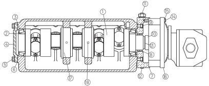
Crankshaft Assembly 2-3/4" Stroke; Auburn Planetary #8
