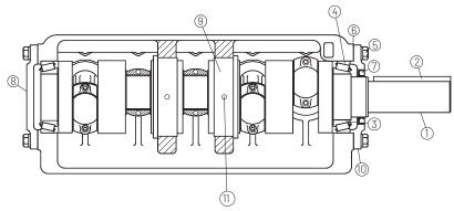
Crankshaft Assembly 2-3/4" Stroke; Right-Hand and Left-Hand Drive; Right-Hand Shown
