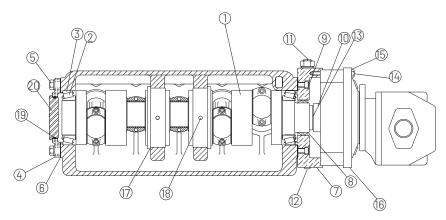
Crankshaft Assembly 2-3/4" Stroke; Auburn Planetary Gear #6
