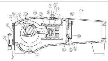
Power Frame Assembly; Connecting Rod, Crosshead & Wiper Box Assembly
