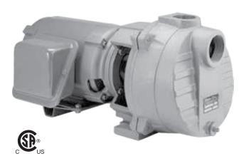
The Quick Prime Self-Priming Centrifugal Pump delivers strong dependable performance for demanding jobs where a lot of water is required over a long period of time. The heavy duty 184JM motor, brass impeller, and large capacity rugged cast iron pump end deliver reliable and continuous high performance service. Not for use with corrosive chemicals or flammable liquids.
