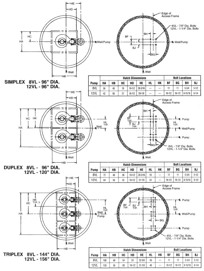
**INSTALLATION, 8VL DUPLEX, 96" DIAMETER WELL, REMOTE**
